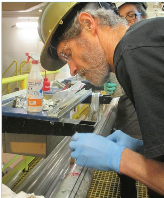
Taking a microbiology sample from a core on the catwalk
