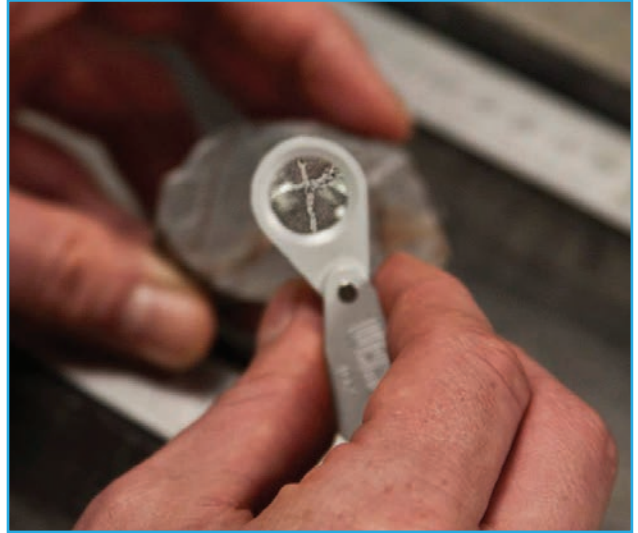
Using a hand lens to examine a vein
