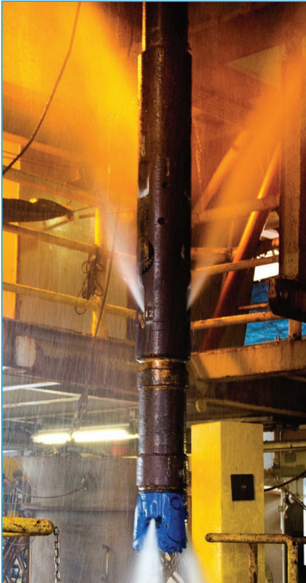
Testing the underreamer
