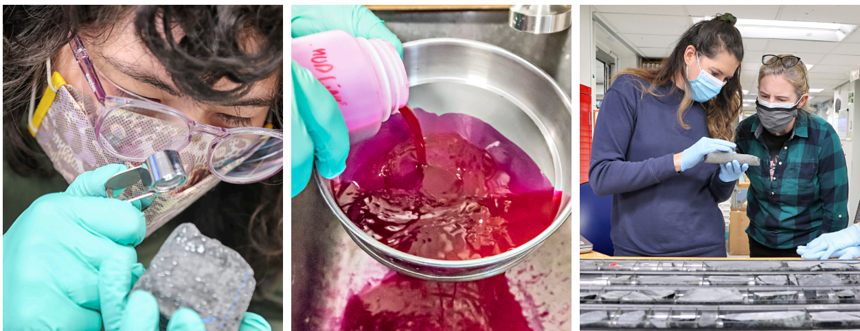
From left: Observing a basalt piece with a hand lens. Soaking a mudline sample in an ethanol-stain mix. Selecting basalt samples for thin sections.
