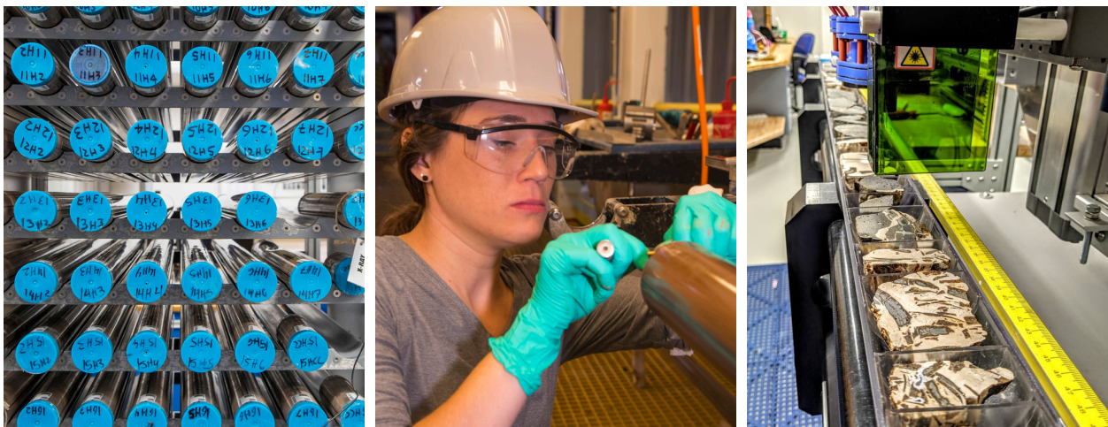
From left: A full core rack waiting for core logging and splitting. Collecting a headspace sample from the lower part of the core. Measuring a hard rock section half in the Section Half Multisensor Logger (SHMSL).
