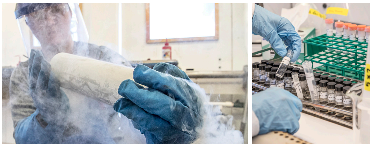
From left: Retrieving a frozen microbiology sample from the liquid nitrogen carrier. Preparing samples for inductively coupled plasma–atomic emission analysis (ICP-AES) analysis.
