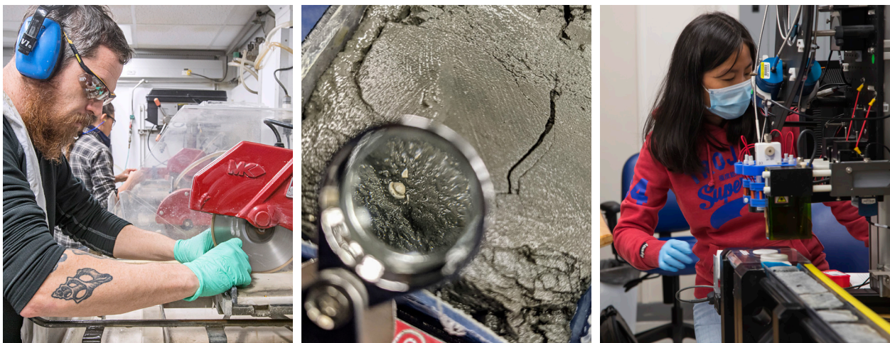
From left: Sawing a piece of hard rock core to create working and archive halves. Using a hand lens to observe a benthic foraminifer sticking out of the mud. Running the Section Half Multisensor Logger (SHMSL).
