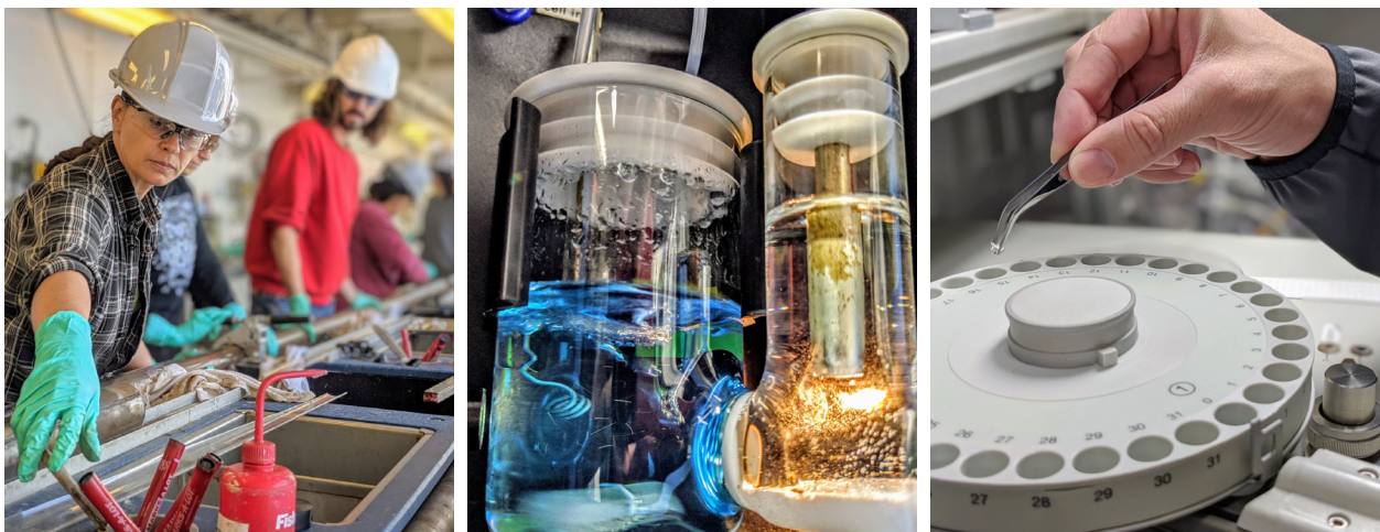
From left: Preparing cores for cutting into sections on the catwalk. Close-up of the coulometer cell after an analysis. Loading samples into the CHNS autosampler.
