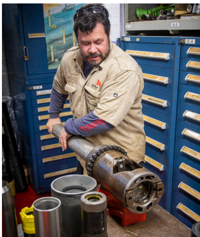
From left: Demonstrating the lockable float valve (LFV) that allows the to return to coring following logging. This technology was developed by IODP. Working at the stratigraphic correlation workstation.
