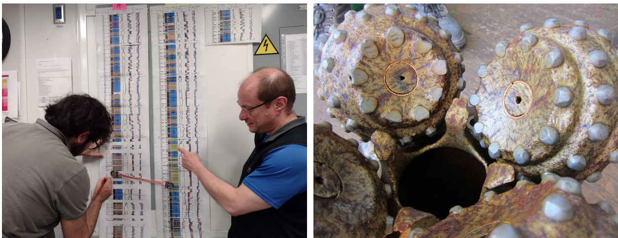
From left: Working on the big picture. Rotary core barrel drill bit after several hours of drilling young basalt.
