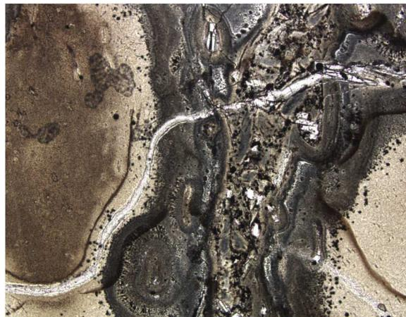
**Figure F102.** Close-up photograph of an anhydrite-pyrite vein (at 76 cm) with a wide halo of bleaching, overprinting an earlier vein network of anhydrite-silica-clay veins, which crosscut pervasively GSC altered volcanic rocks (Sample 193-1188A-12R-1 [Pieces 7–8, 71–90 cm]; 97.17 mbsf).
