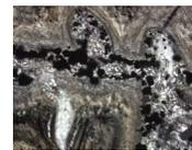
F43. Quartz-pyrite veining with well-developed silica-chlorite alteration halos, p. 146.
