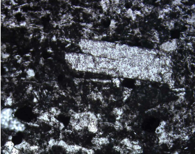
**Figure F53.** Anhedral former magnetite microphenocryst, which has broken down to leucoxene (dark patch in central portion of image), with remnant trellislike laths of magnetite faintly visible. A pyrite cube overgrows the magnetite (interval 193-1188A-19R-1, 73–76 cm, Unit 19, in reflected light; width of view = 0.7 mm. Photomicrograph ID# 1188A\_93; **thin section 21**).
