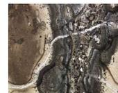
F72. Veins of anhydrite and pyrite together with disseminated pyrite in highly altered dacite, p. 175.
