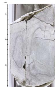
Unit 30 is a brecciated volcanic rock with silicified fragments embedded in a light gray clay-rich matrix (Fig. F22). This texture, though, may be a drilling-induced characteristic of the ADCB system because most of the recovered pieces consist of rubble. The fine, soft, clay-rich material may be an artifact caused by the grinding.
