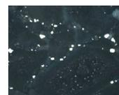
F74. Subhedral pyrite containing vermicular inclusions of magnetite, p. 177.
