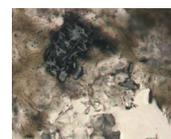
[F78](#). Subhedral Fe-rich sphalerite precipitated on euhedral pyrite in a cavity, p. 181.
