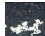
F94. Euhedral quartz overgrown by a second quartz containing inclusions of magnetite in turn overgrown by pyrite, p. 197.
