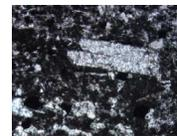
F53. Anhedral former magnetite microphenocryst with remnant trellislike laths of magnetite faintly visible, p. 156.
