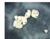
F92. Magnetite inclusions in pyrite having the same morphology as those in the neighboring quartz in the groundmass, p. 195.
