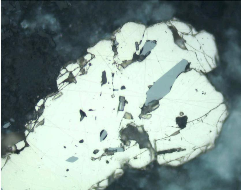
Figure F85. Chalcopyrite (yellow) partially replacing pyrite (white) (Sample 193-1188F-37Z-2 [Piece 3, 31–33 cm] in reflected light; width of view = 0.28 mm. Photomicrograph ID# 1188F\_109; **thin section 101**).
