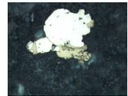
F86. Ti magnetite with ilmenite exsolution laths, p. 189.
