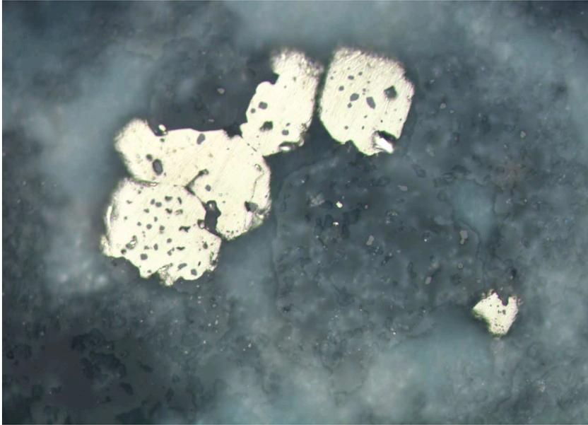
**Figure F92.** Magnetite (gray) inclusions in pyrite (white) having the same morphology as those in the neighboring quartz (black) in the groundmass. Magnetite inclusions in the center of the pyrite grain are smaller than those near the edge suggesting that the former have been partially replaced (Sample 193-1188F-25Z-1 [Piece 4, 24–26 cm] in reflected light; width of view = 0.275 mm. Photomicrograph 1188F\_71).
