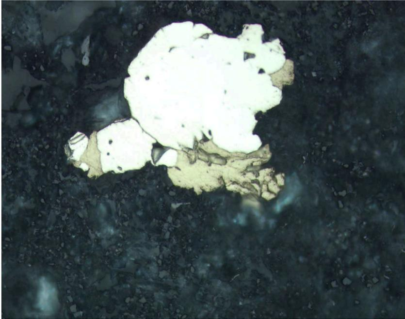
Figure F86. Ti magnetite with ilmenite exsolution laths (Sample 193-1188F-30Z-1 [Piece 2, 5–7 cm] in reflected light; width of view = 0.14 mm. Photomicrograph ID# 1188F\_65; [thin section 91](#)).
