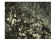
F61. An apparently spherulitic unit, showing spherical domains in a cristobalite-clay matrix, p. 164.
