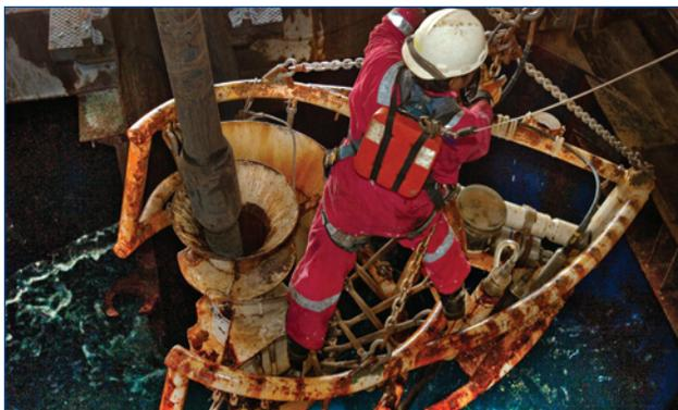
Connecting underwater camera to a crane for retrieval from the moonpool
