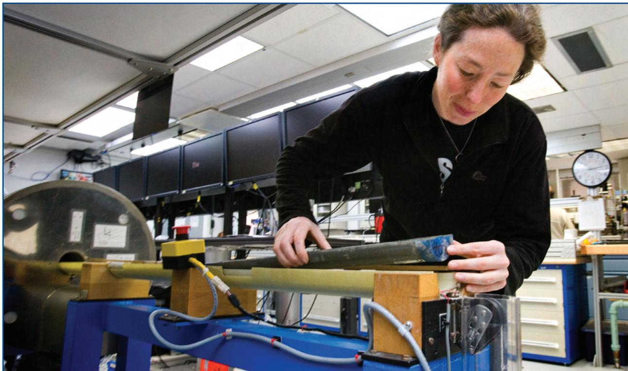
Measuring a core section with the cryogenic magnetometer
