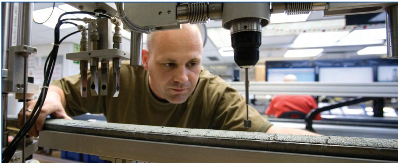
*Measuring shear strength of sediment*
