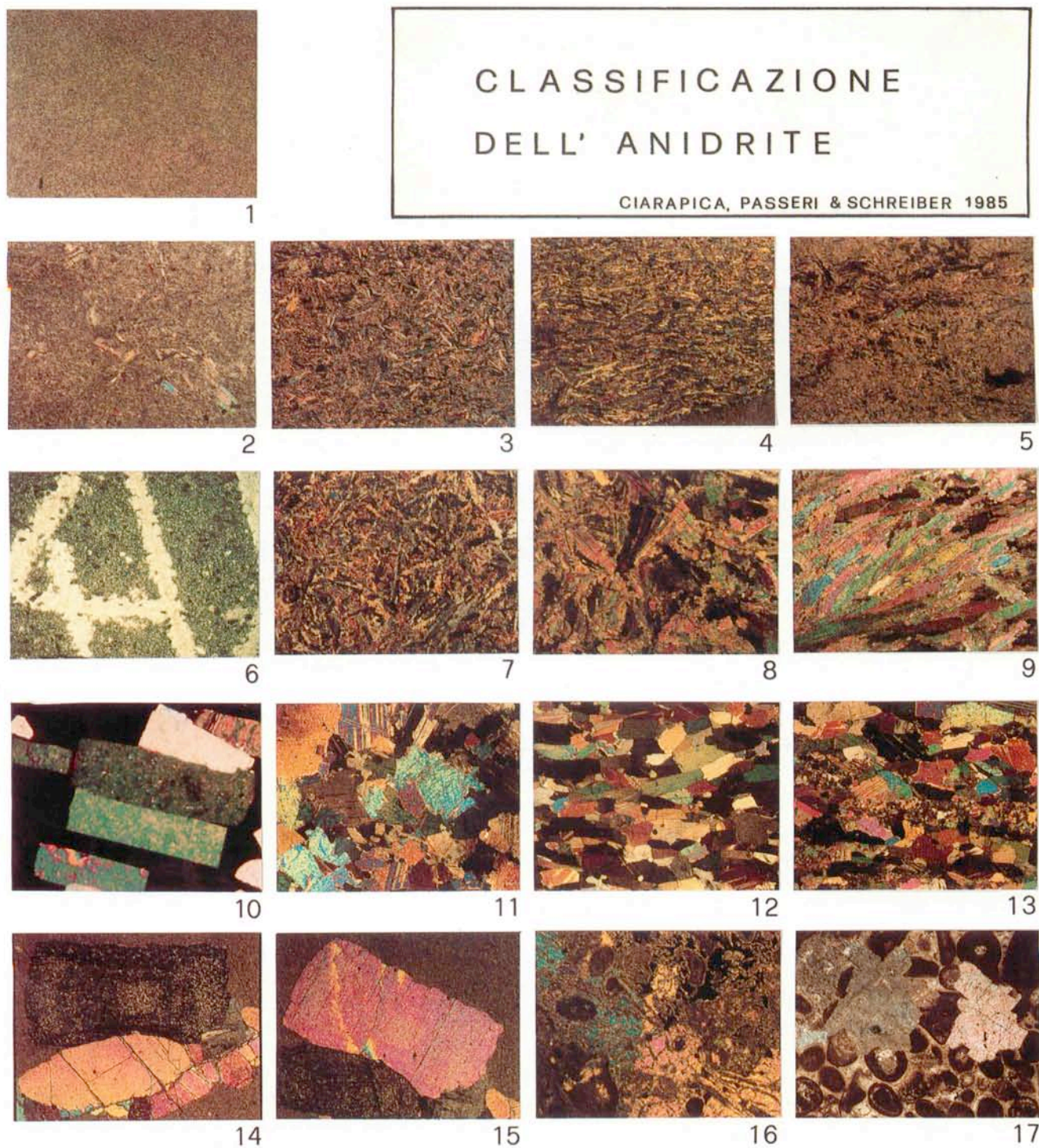
FIG. 2 — 1 - MICROCRYSTALLINE ANHYDRITE (crystal size < 0,06 mm); 2-5: FELTED ANHYDRITE (acicular crystals < 0,5 mm); 2- SUBFELTED ANHYDRITE (acicular crystals < 0,5 mm + microcrystals); 3- FELTED ANHYDRITE (non oriented crystals); 4- ALIGNED-FELTED ANHYDRITE (isooriented crystals); 5- STREAKED-FELTED ANHYDRITE (acicular crystals, often aligned, with streaks made up by fragments of non sulfate material); 6-9: FIBROUS ANHYDRITE (lath-shaped crystals > 0,5 mm); 6- FIBROUS SCATTERED ANHYDRITE (scattered crystals in non sulfate matrix); 7- INTERSECTING FIBROUS ANHYDRITE (non oriented crystals); 8- RADIAL FIBROUS ANHYDRITE (crystals in aggregates, with radial orientation); 9- ALIGNED FIBROUS ANHYDRITE (aligned crystals); 10-13: PRISMATIC ANHYDRITE: 10- NON ORIENTED PRISMATIC ANHYDRITE (non oriented crystals); 11- GRANULAR PRISMATIC ANHYDRITE (non oriented prismatic crystals with sutured boundaries); 12- ALIGNED PRISMATIC ANHYDRITE (aligned prismatic crystals); 13- STREAKED PRISMATIC ANHYDRITE (prismatic crystals, often aligned, with streaks made up by fragments of non sulfate material); 14-15: AXE-HEADED ANHYDRITE (axe-headed crystals often zoned); 16-17: PATCH ANHYDRITE (anhydrite patches in a non sulfate sediment); 16- AMEBOID PATCH ANHYDRITE (irregular patches); 17- STAIR-STEPS ANHYDRITE (patches with angular boundaries).
