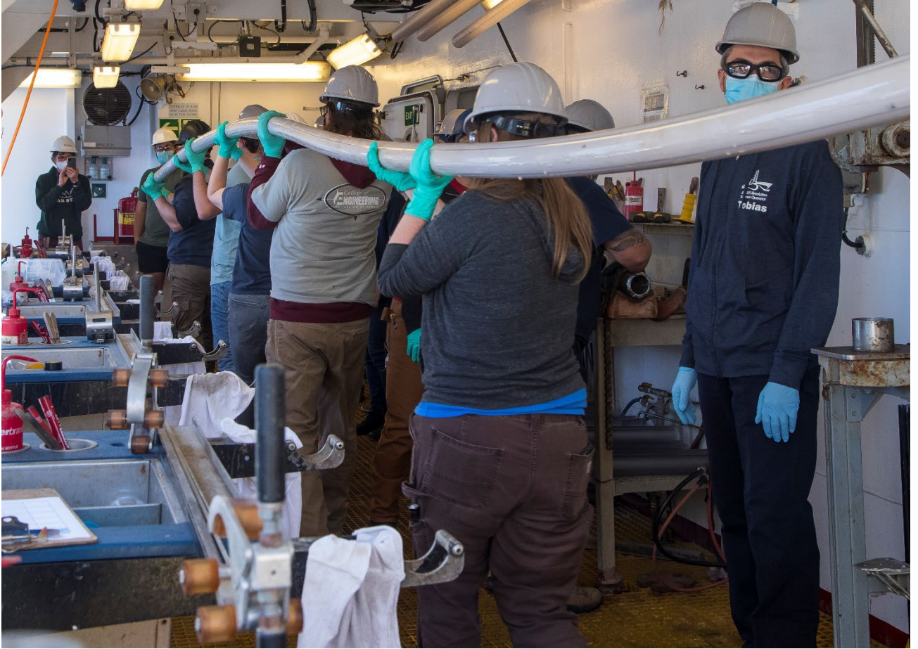
Figure 1. Core being carried to the catwalk from the rig floor.
