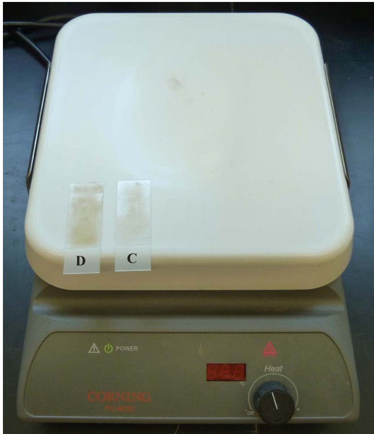
Figure 5. Smear slides are then placed on a moderately heated hot plate to dry. It is important to leave the labeled end off the plate surface to facilitate removal of the hot dried slide.
