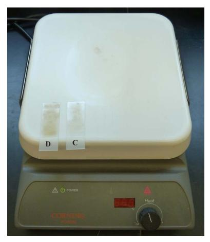
Figure 6. Smear slides are placed on a moderately heated hot plate to dry. It is important to leave the labeled end off the plate surface to facilitate removal of the hot dried slide.
