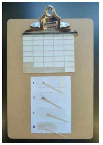
Figure 5. With muddy sediments the amount of material needed is small, just covering the end of a toothpick. Two amounts are shown, one smaller (c) and one larger (d), with the latter wetted and in the process of disaggregation. The amount of material determines the consistency of the slurry, whether it is more dilute (C) or more dense (D), which in turn affects the petrographic analysis. The material can be too thinly or too thickly spread. See Slide Tutorials for examples.
