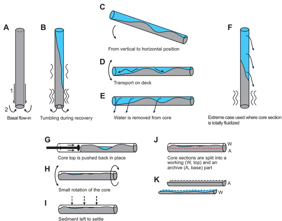
**Figure F4.4.** Diagram showing how “soupy” texture can also be produced by sloshing of water and sediment in partly filled core liners extracted from the core barrel and laid horizontal on the catwalk (from Jutzeler et al., 2014).
