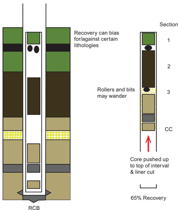
**Figure F4.2.** Schematic of rotary-drilled core recovery considerations and formation. RCB = rotary core bit.
