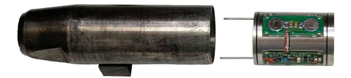
APCT-3 shoe (left) has a pocket to accept electronics, memory board, and battery (right) for temperature measurements while taking an APC core.
