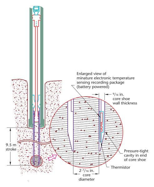
Continuous temperature measurements are recorded with the APCT core shoe embedded in the sediment.
