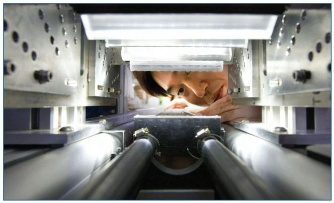
Inserting a core section into the imaging logger
