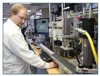
Taking discrete measurements from a core section
