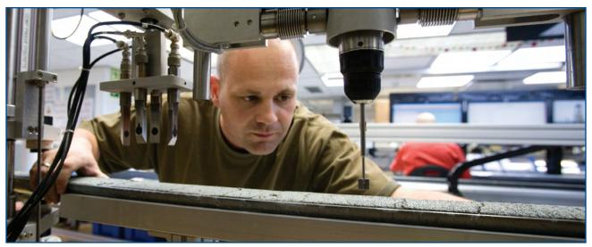
Measuring shear strength of sediment
