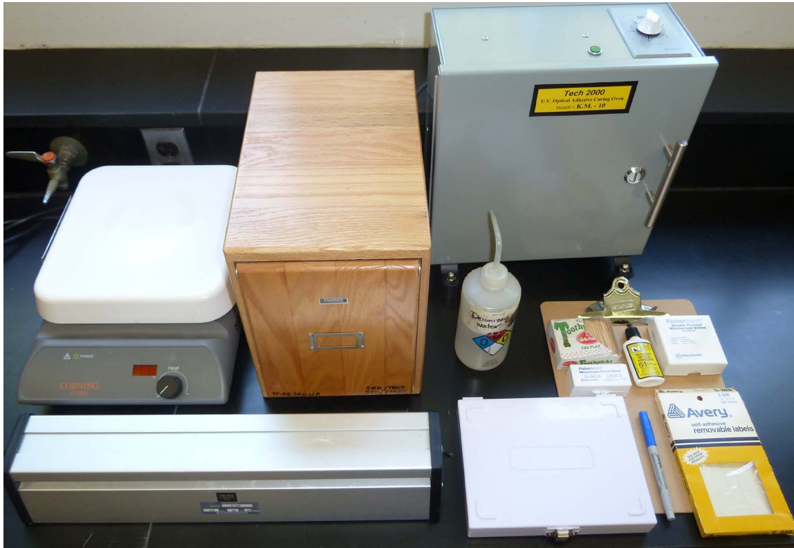
Figure 3. The equipment needed for smear slide preparation includes a hot plate (A); UV curing apparatus, either a UV light (B) or specially manufactured box (D); slide storage, such as wood benchtop box with trays (C) or plastic portable box (F); water bottle (E), preferably with nanopure water if available; flat toothpicks (G); slide coverslips (H); optical adhesive (I) such as Norland 61; glass slides (J); slide labels (M); and a permanent fine-point marker (L). Note that shipboard slide labels are automatically generated with barcodes. Shore-based slides can be marked with adhesive labels, but these may ultimately deteriorate. If glass slides with frosted ends are used, slide information can be written directly on the slide with a permanent fine-point marker.
