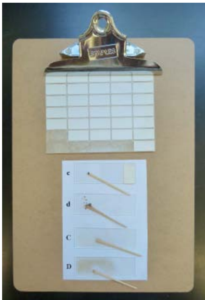
Figure 4. With muddy sediments the amount of material needed is small, just covering the end of a toothpick. Two amounts are shown, one smaller (c) and one larger (d), with the latter wetted and in the process of disaggregation. The amount of material determines the consistency of the slurry, whether it is more dilute (C) or more dense (D), which in turn affects the petrographic analysis. The material can be too thinly or too thickly spread. See Slide Tutorials for examples.
