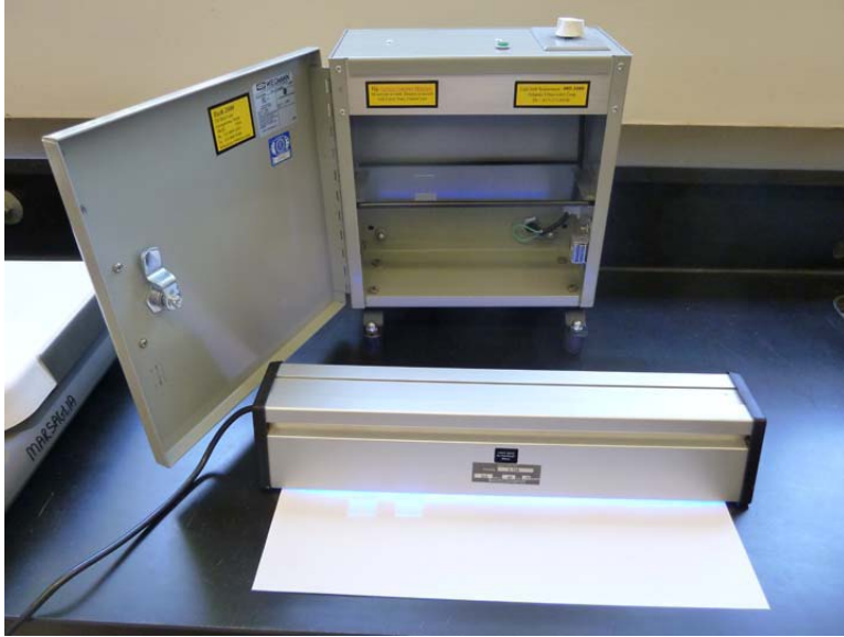
Figure 7. UV light curing apparatuses also pictured in Figure 3. Purple to bluish glow signals the lamps are switched on (note that you should avoid directly viewing UV light). Slides are placed on a tray or piece of paper to cure either under a UV lamp or within a specially made curing oven. The UV lamp, a less expensive option, can simply be placed over the slides as pictured here. The length of time needed to fully cure is normally less than 10 minutes but may vary. A simple touch of the finger can test whether extruded adhesive is tacky (partly cured) or fully solidified (cured).
